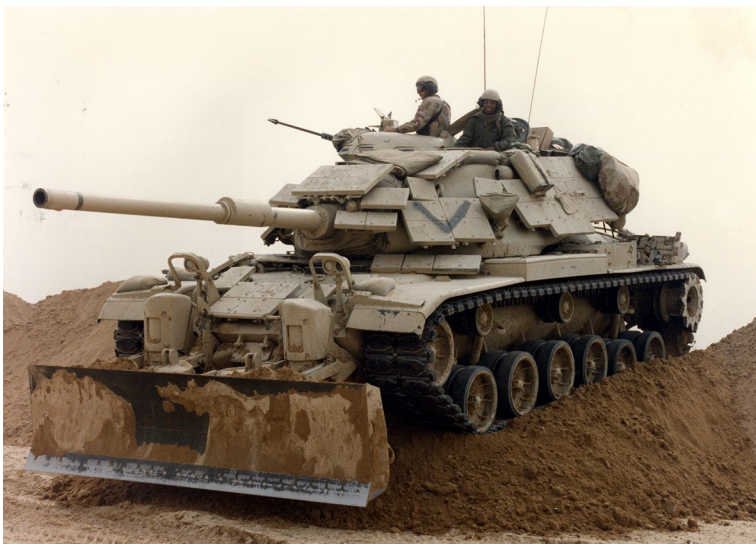
Marines from Company D, 2d Tank Battalion, drive their M60A1 main battle tank during a breach exercise in Operation Desert Storm in 1991. The tank is fitted with reactive armor and an M-9 bulldozer kit. (USMC Photo)
